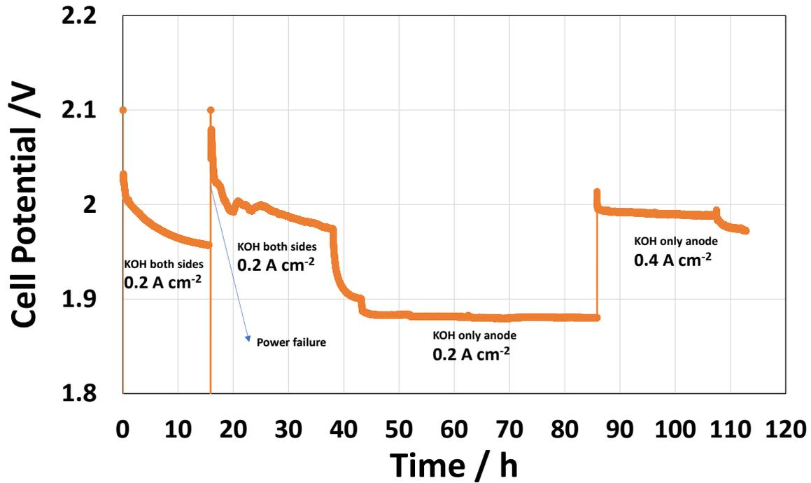
**Figure 39.** Durability test conducted under galvanostatic conditions (i.e. 0.2 A cm<sup>-2</sup>- 0.4 A cm<sup>-2</sup>) for the cell based on Ni<sub>0.4</sub>Cu<sub>0.4</sub>Mo<sub>0.2</sub> as cathode and NiFe oxide as anode at 50 °C and by feeding KOH on both sides of cell.
