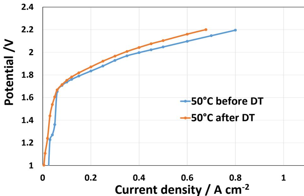
**Figure 41.** Comparison of polarization curves at the beginning and end of the Durability test (conducted under galvanostatic conditions) at 50 °C with the cell based on Ni<sub>0.4</sub>Cu<sub>0.4</sub>Mo<sub>0.2</sub> as cathode.
