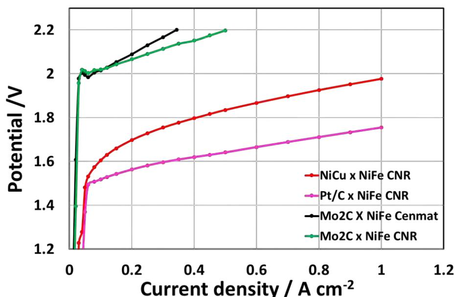
**Figure 42.** Comparison of polarization curves at 50 °C with the cell based CNR-ITAE catalysts and the cell based commercial catalysts.
