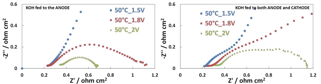
**Figure 38.** The EIS of cell based  $\text{Ni}_{0.4}\text{Cu}_{0.4}\text{Mo}_{0.2}$  as cathode and NiFe oxide as anode measured at 50 °C by feeding KOH at one or both sides of cell.
