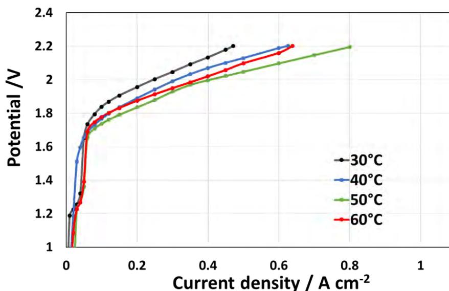
**Figure 35.** Comparison of polarization curves carried out on the cell mounting  $\text{Ni}_{0.4}\text{Cu}_{0.4}\text{Mo}_{0.2}$  as cathode and NiFe oxide as anode in the temperature range 30 °C - 60 °C.
