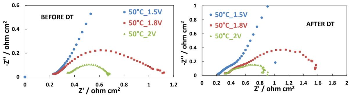
**Figure 40.** The EIS of cell based  $Ni_{0.4}Cu_{0.4}Mo_{0.2}$  as cathode and NiFe oxide as anode measured at 50 °C by feeding KOH after durability test.
