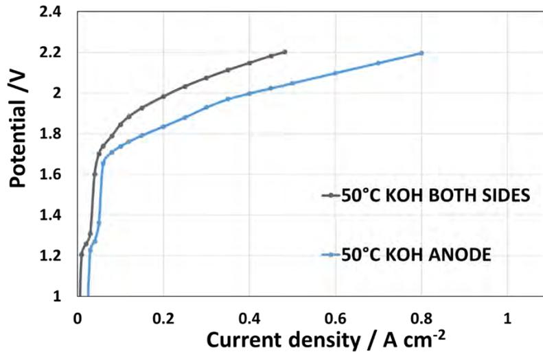
**Figure 37.** A comparison of polarization curves carried out on the cell based  $\text{Ni}_{0.4}\text{Cu}_{0.4}\text{Mo}_{0.2}$  as cathode and NiFe oxide as anode at 50 ° by feeding KOH on one or both sides of cell.
