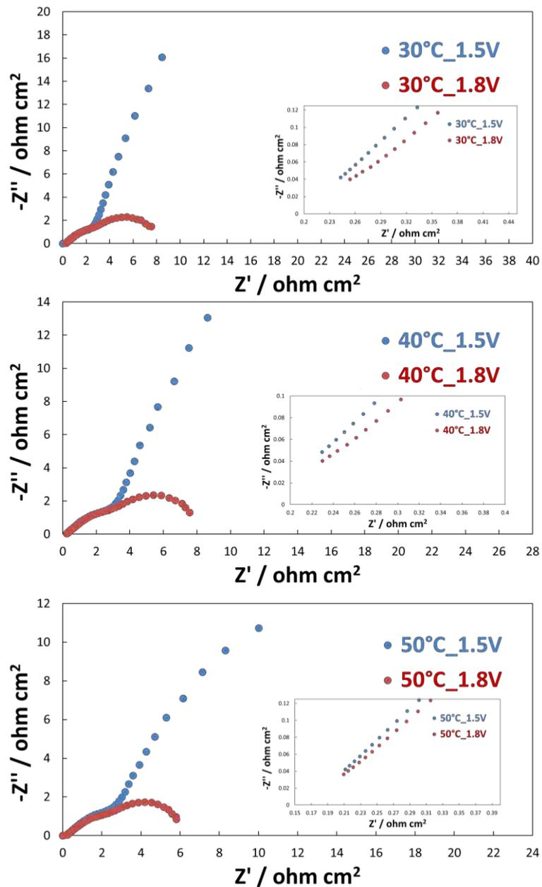
**Figure 33.** The EIS of cell based on NiMo as cathode and NiFe oxide as anode measured at 1.5 V and 1.8 V at 30 °C (a), 40 °C (b) and 50 °C (c).
