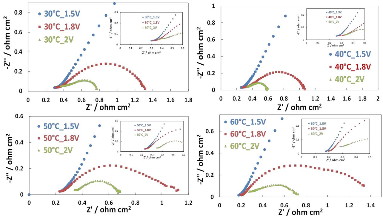
**Figure 36.** The EIS of cell based on  $\text{Ni}_{0.4}\text{Cu}_{0.4}\text{Mo}_{0.2}$  as cathode and NiFe oxide as anode measured at 1.5 V and 1.8 V at 30 °C (a), 40 °C (b), 50 °C (c) and 60 °C (d).
