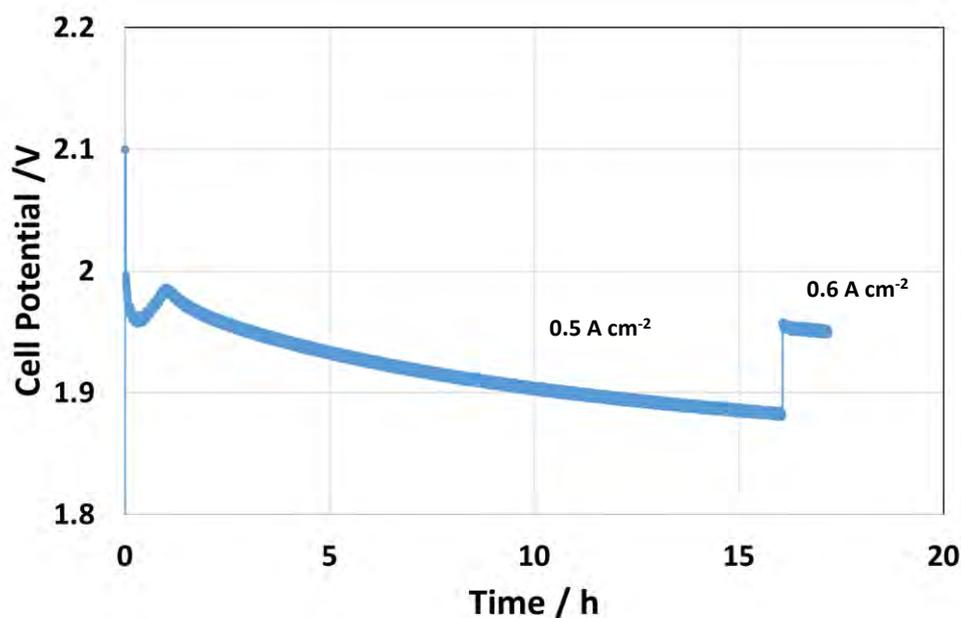
**Figure 34.** Durability test carried out under galvanostatic conditions at 50 °C for cell based on NiMo as the cathode and NiFe oxide as anode.
